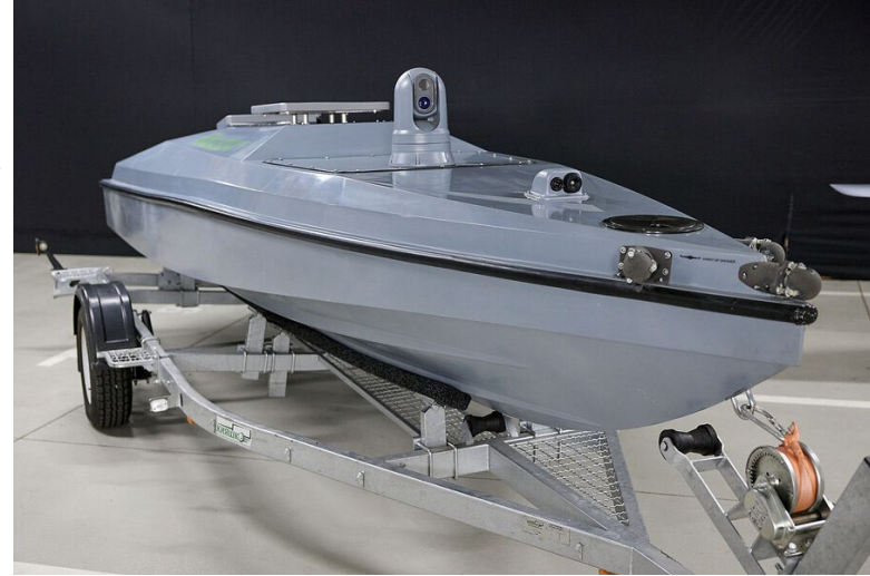
A Magura V5 (maritime autonomous guard uncrewed robotic apparatus V-type), a Ukrainian multipurpose uncrewed surface boat, or sea drone, is seen in Ukraine.
